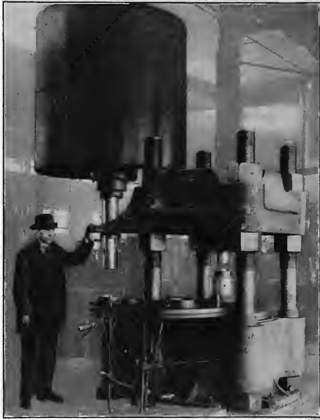
FIG. 2. ANGUS-BUILT CARTRIDGE-HEADING PRESSES AND ACCUMULATORS TO OPERATE THEM
